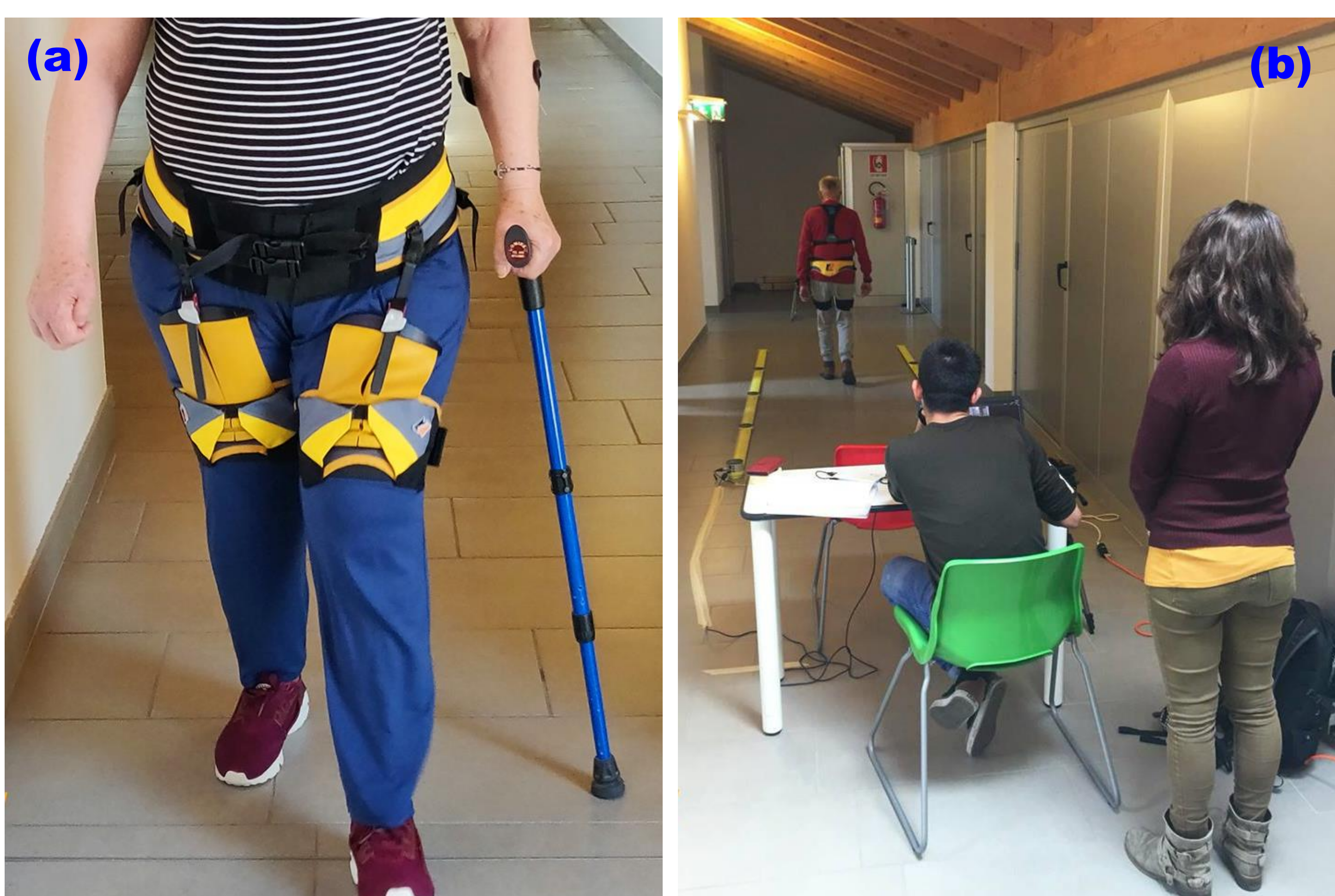
Fig. 1 (a) Exoband worn by a patients during testing (b) Testing setup of day 2.
